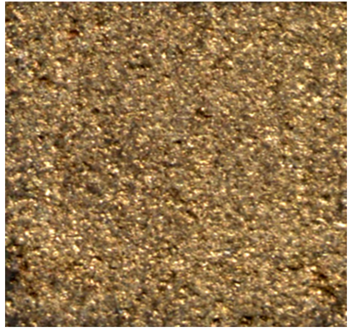
Figure 16. General view of the surface layer obtained by the method of metallic powder deposition using pulsed discharges with contact break (Cathode – Steel 45; Anode – BrOTS-5-5-5; Metallic powder – BrA-7; Magnification \times 20 .)
